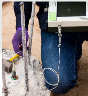
Pile Integrity Test
