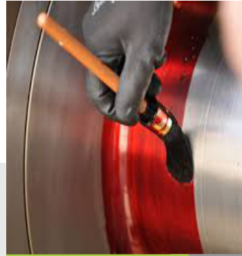
Liquid Penetrant Testing
