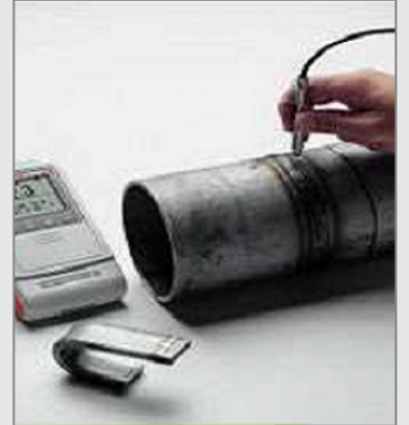
Eddy Current Inspection
